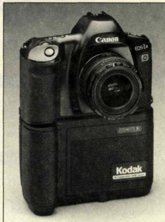
Kodak and Canon combined to produce the EOS * DCS 5, a $12,000 pro digital camera based on the Canon EOS-1n pro AF SLR body.
