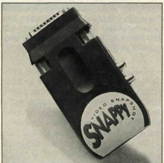
The Snappy Video Snapshot does what its name suggests—captures still images from video sources (TV, VCR, camcorder, etc.) so you can use them in your computer.
